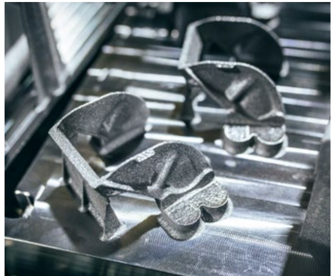
Two proximity sensor brackets for the Airbus A350 nose landing gear after the printing process
