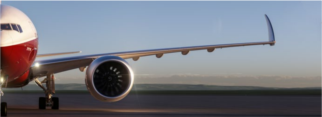
The Boeing 777X will be equipped with Liebherr-Aerospace's technology for the folding wing tip system – making it the first commercial airliner in history with folding capabilities
