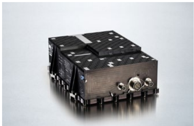
Slat actuation electronic control unit for the Airbus A350 program
