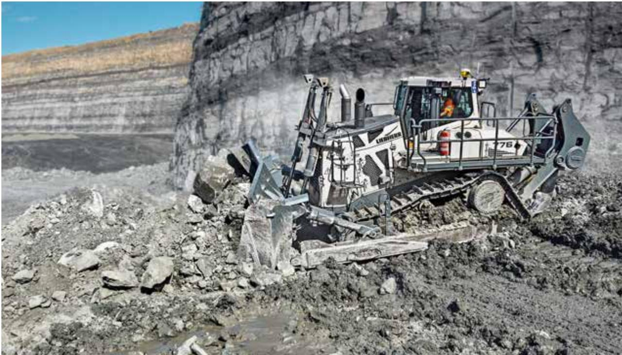
At the Bauma trade fair in Munich (Germany), Liebherr presented the PR 776, the world's largest crawler tractor with an infinitely variable hydrostatic drive. The PR 776 has been specially designed to operate under the toughest mining and extraction conditions. The first units are in operation in Russia, Australia and the USA.
