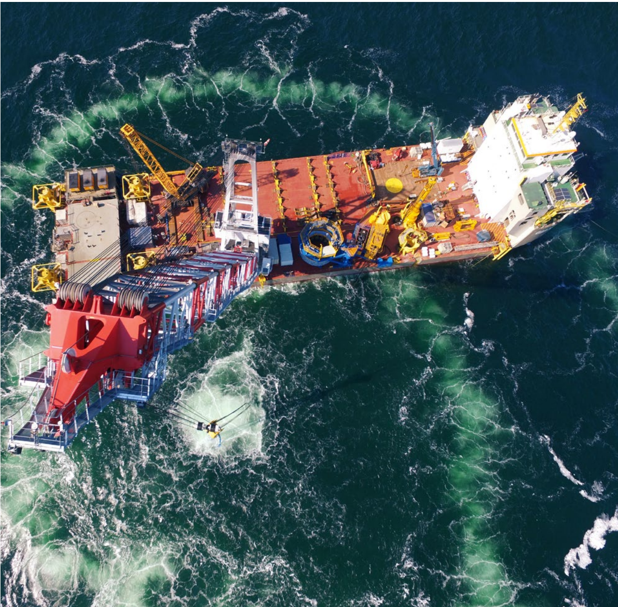
An offshore crane, type BOS 35000, installs a wind farm in the Baltic Sea
