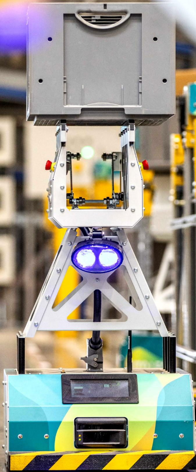
Driverless transport systems carry small parts autonomously in the Liebherr spare parts warehouse in Oberopfingen (Germany)
