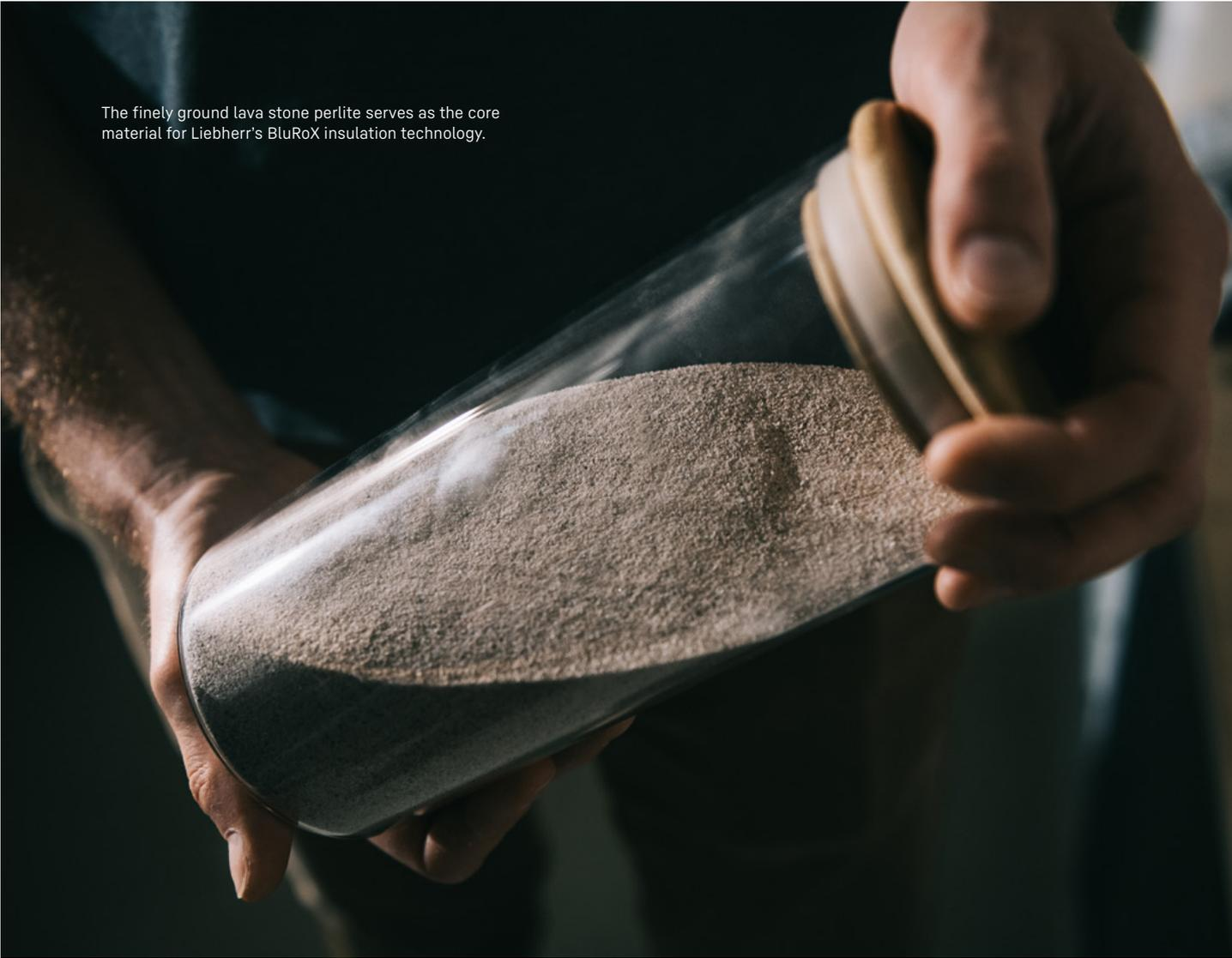
The finely ground lava stone perlite serves as the core material for Liebherr's BluRoX insulation technology.
