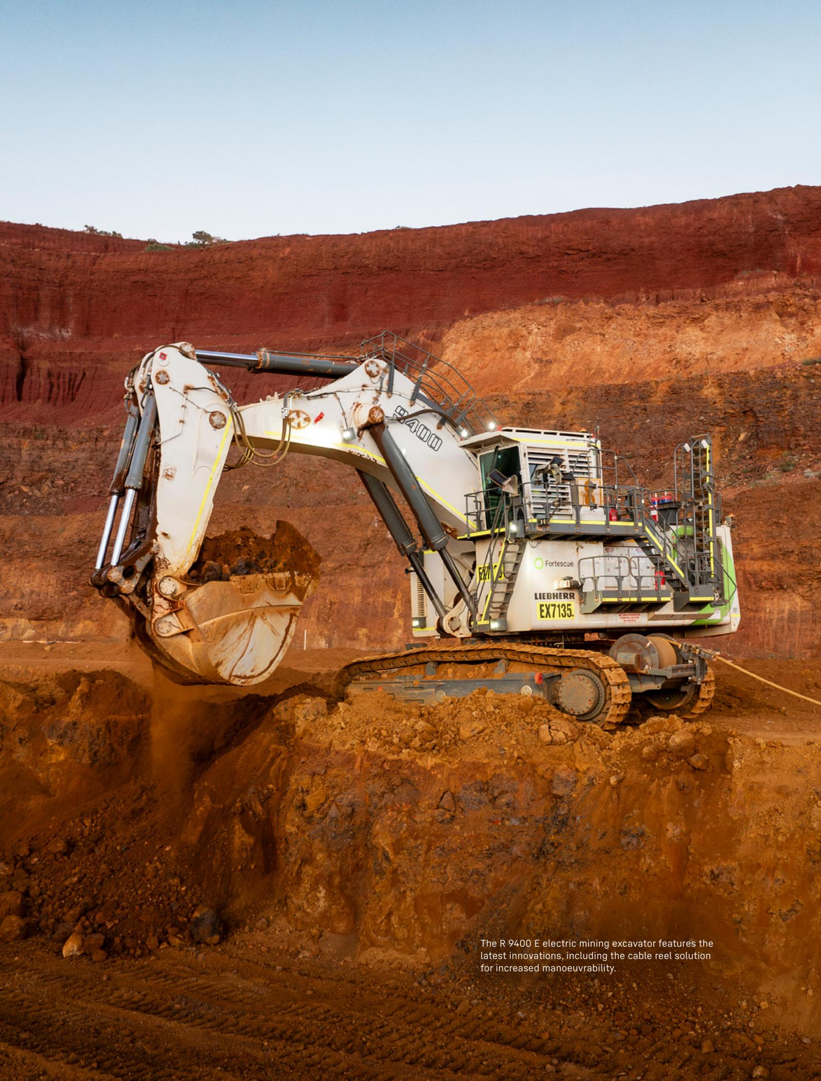
The R 9400 E electric mining excavator features the latest innovations, including the cable reel solution for increased manoeuvrability.
