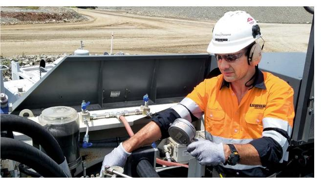
Measuring valve pressure on a new machine
