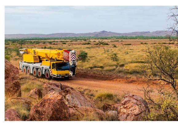
in this size category, the LTM 1160-5.2 has only one engine with mechanical shaft drive.
