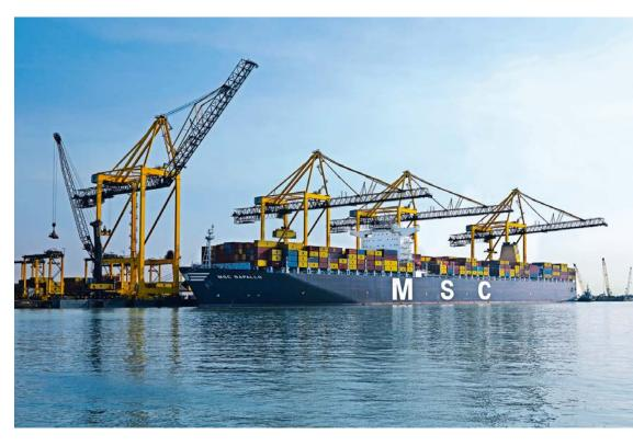
Liebherr configured special container handling gantries for a customer in Australia. In order to comply with height restrictions imposed by the nearby Sydney airport, three container cranes were equipped with articulated booms.
