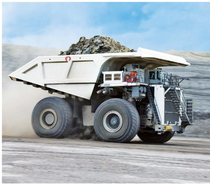
The T 284 mining truck has a gross weight of up to 600 tonnes
