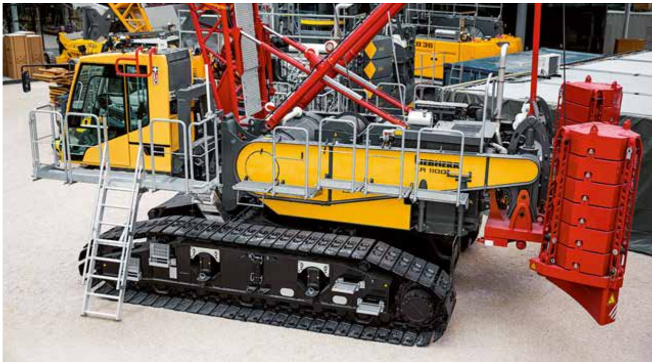
The LR 1100 with its new driver's cabin and swing-out ballast system
