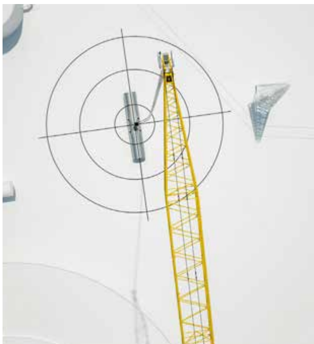
The Vertical Line Finder ensures a perfectly vertical lift
