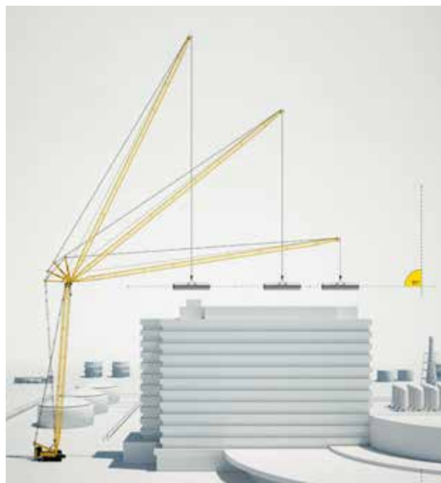
Support for accurate horizontal movements of loads
