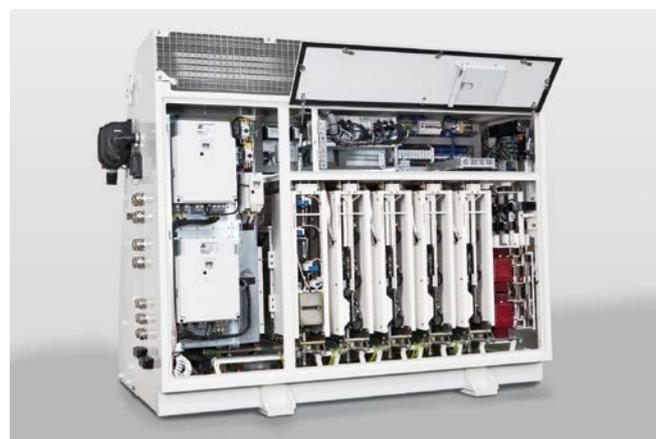
Switchgear cabinet for a mining dump truck
