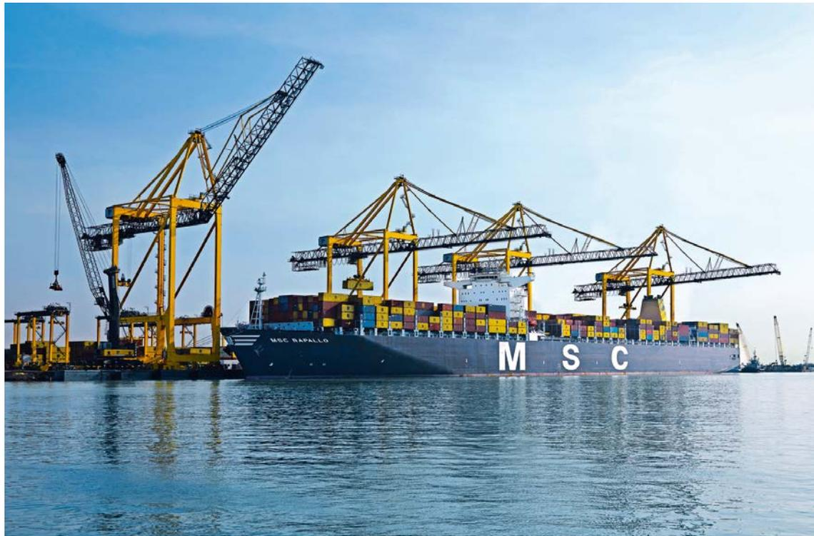
Liebherr configured special container handling gantries for a customer in Australia. In order to comply with height restrictions imposed by the nearby Sydney airport, three container cranes were equipped with articulated booms.
