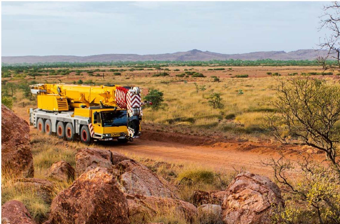
in this size category, the LTM 1160-5.2 has only one engine with mechanical shaft drive.
