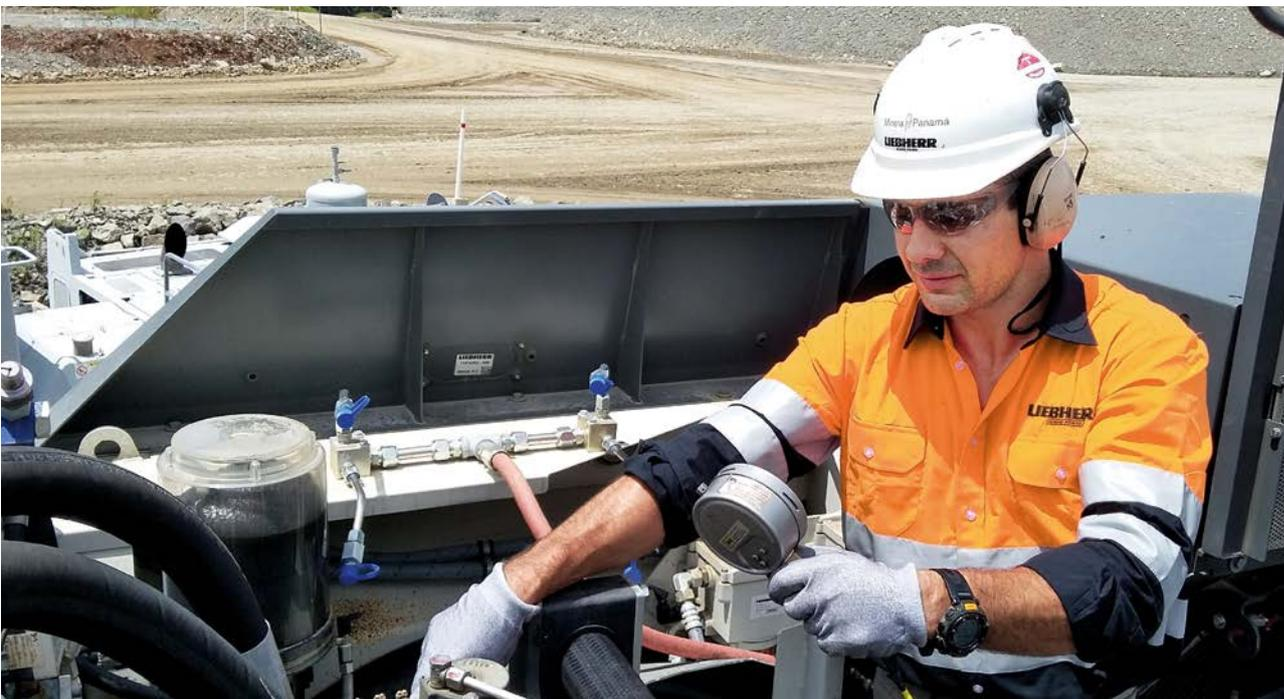
Measuring valve pressure on a new machine
