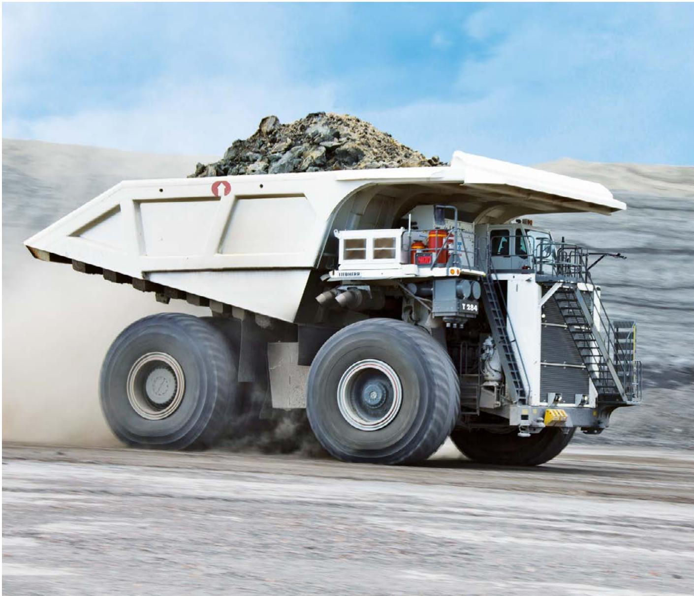
The T 284 mining truck has a gross weight of up to 600 tonnes
