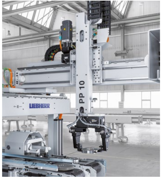
Gantry robot for workpieces with weight between 0.5 kg to 1,500 kg
