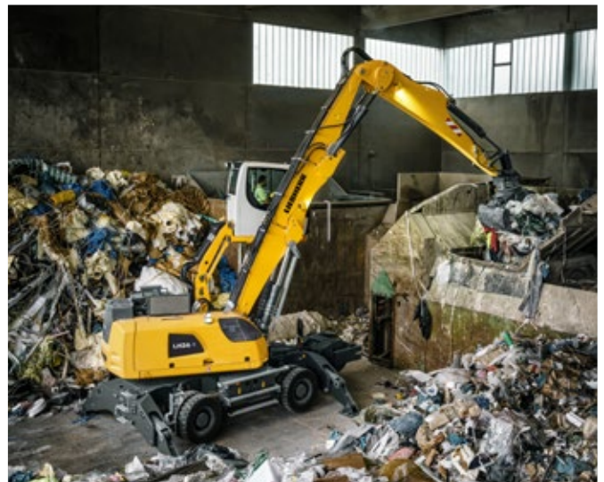
The electric LH 26 M Industry Litronic used in recycling
