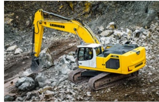
The R 938 crawler excavator in use in a quarry in Metzeral (France)
