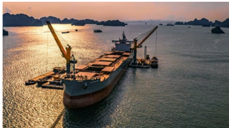
The Liebherr CBG 360 doing dry bulk cargo handling on a transshipment barge in Vietnam
