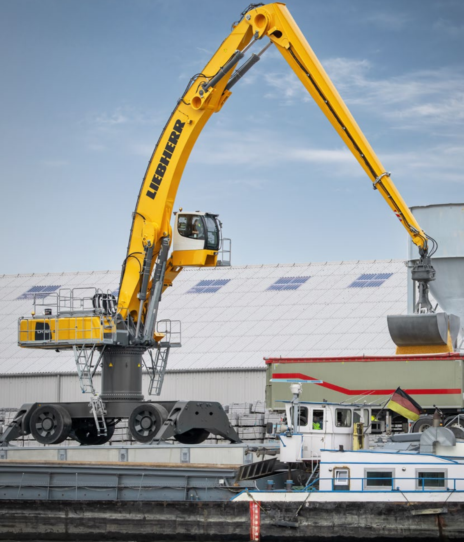
The LH 110 M High Rise Port Litronic used for port handling operations
