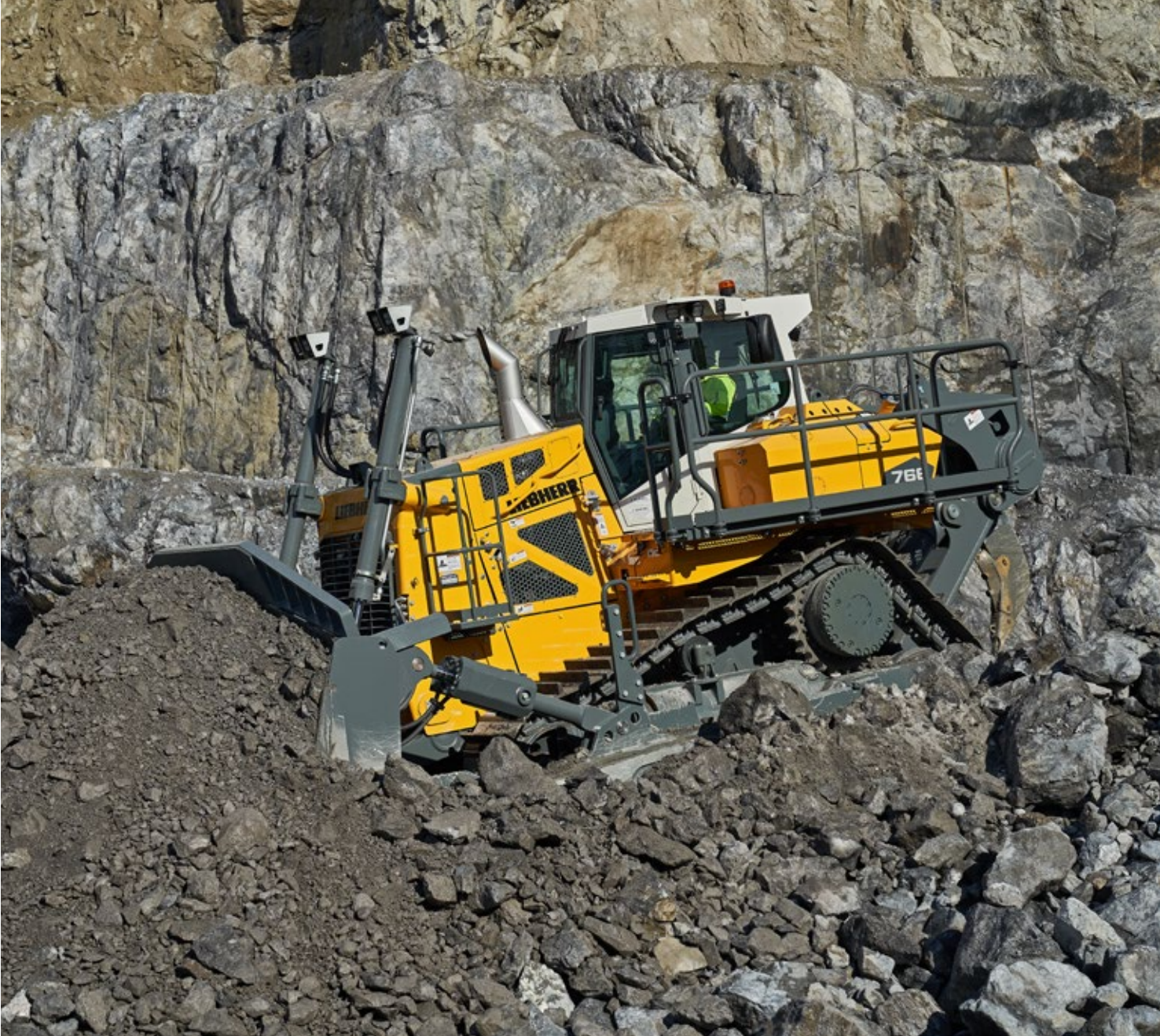
The PR 766 G8 crawler dozer in quarry operations
