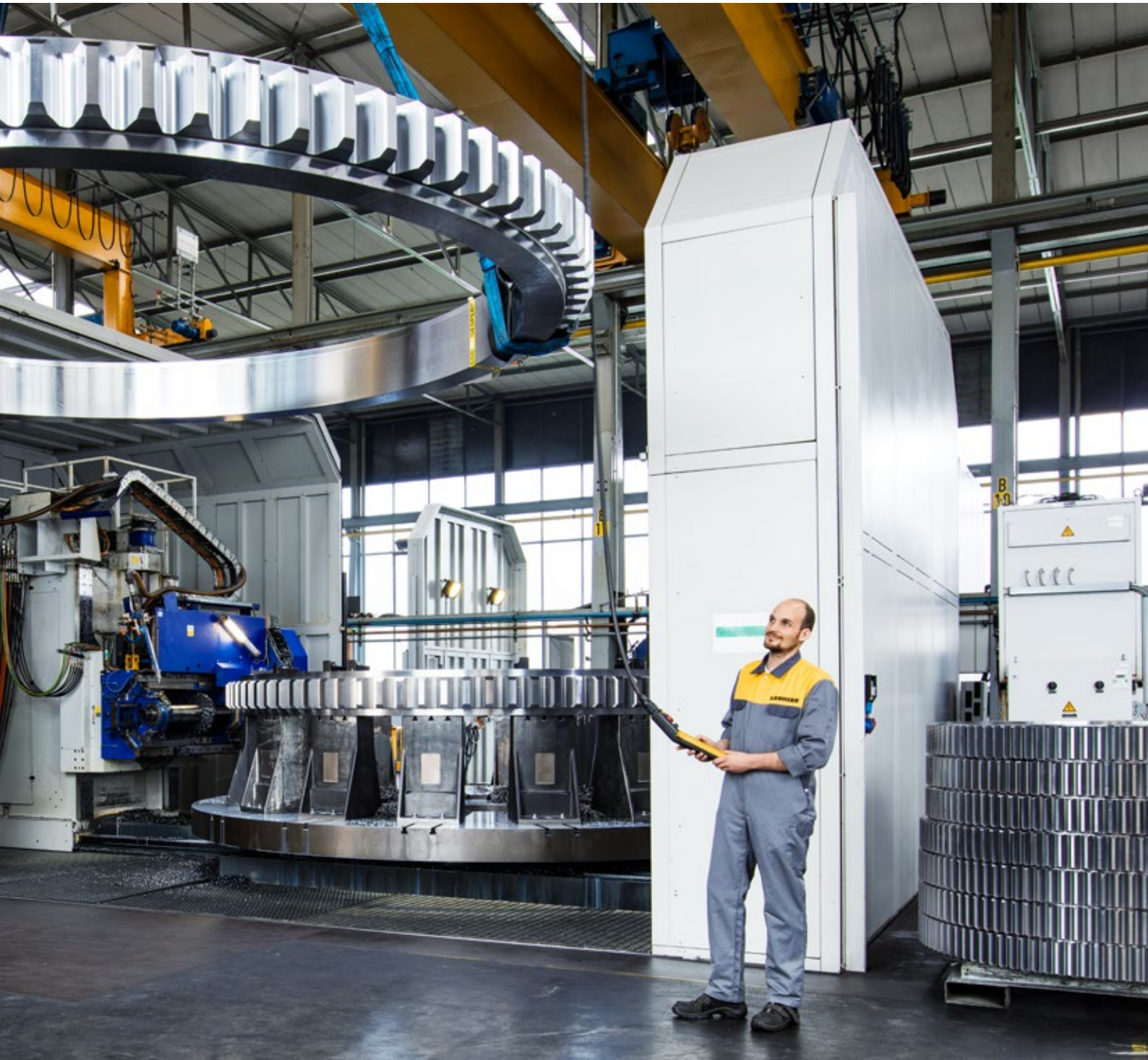
Fine machining through grinding and polishing
