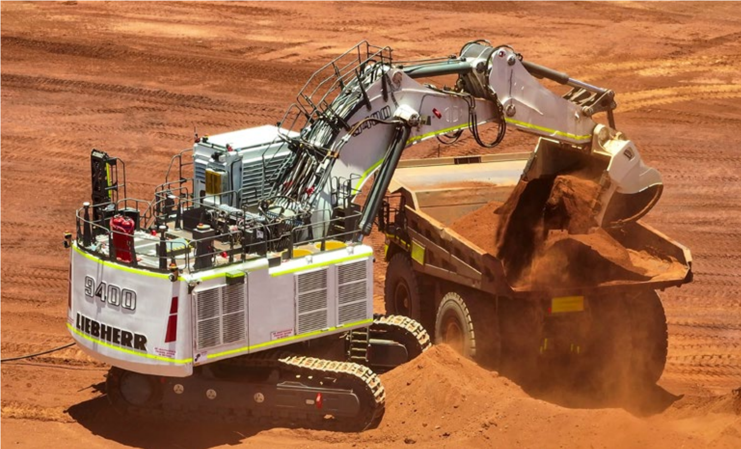
The R 9400 E electric excavator operating in a mine in Australia
