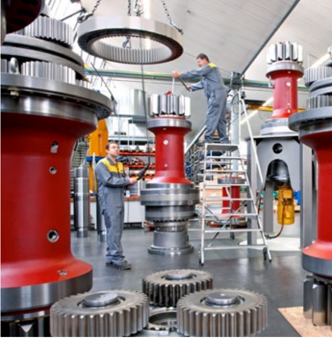
Assembly of DAT 1000 slew drives
