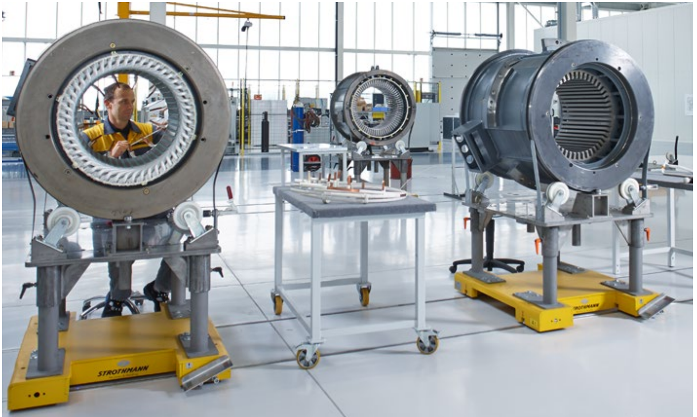
Winding of electric machines for mining trucks and port cranes
