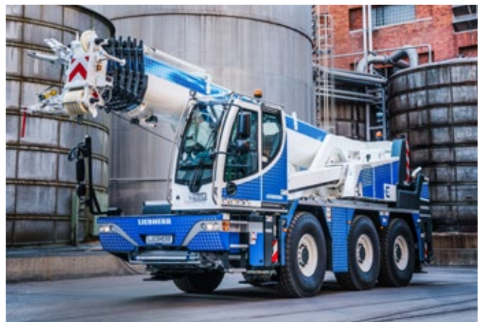
Compact cranes from Liebherr are distinguished by their small size. The hybrid model gives the option of controlling crane movements via an electric motor.
