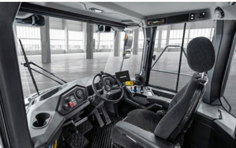
The modern operator's cab of the TA 230 Litronic
