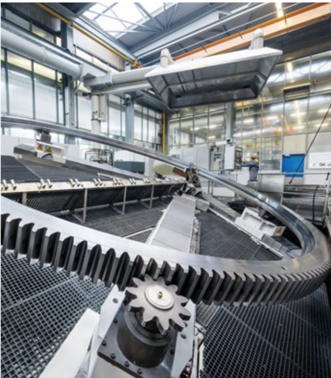
Inductive hardening of slewing bearings
