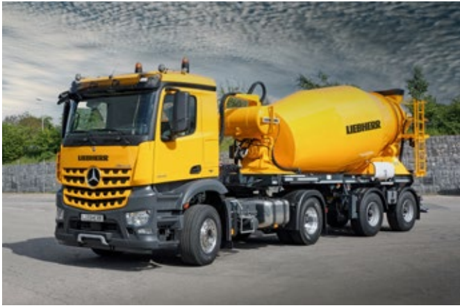
The HTM 1004 ZA/38 truck mixer is approved for a total weight of 38 t.
