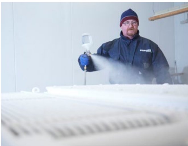
Ice test of an HVAC system
