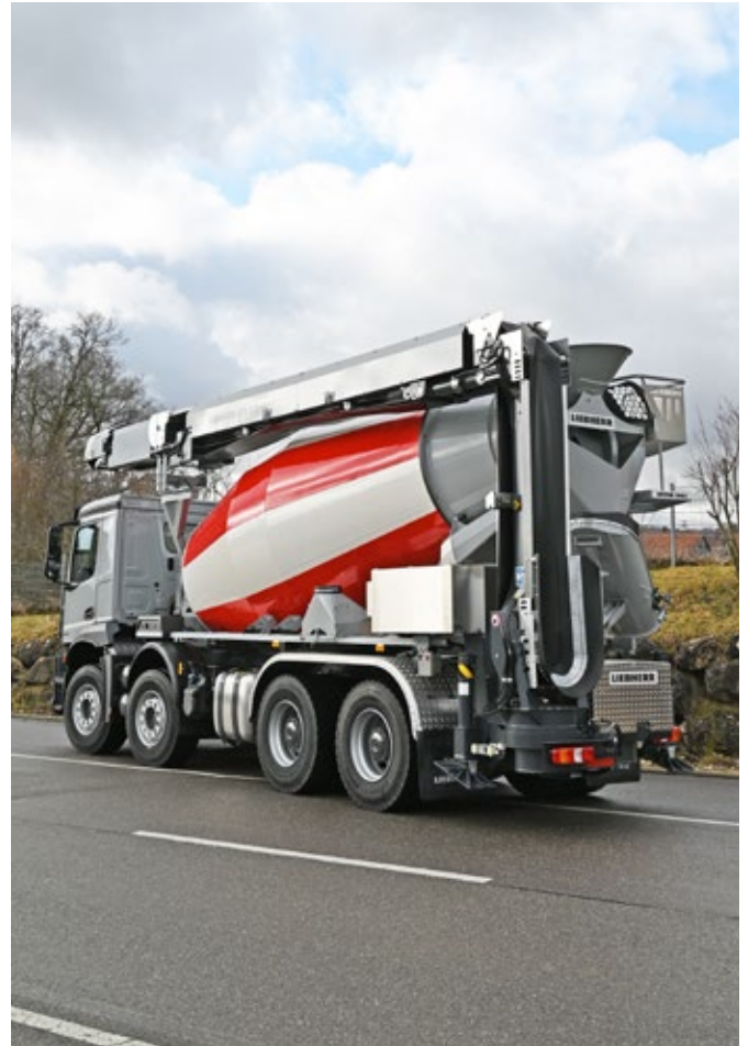
The HTM 1005 truck mixer with LTB 12+4+1 double telescopic conveyor belt
