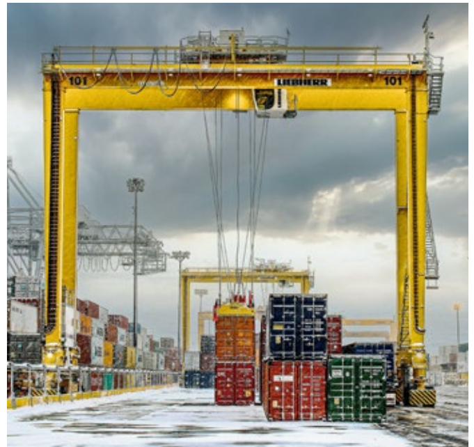
Liebherr electric drive rubber tyre gantry cranes at Montreal Gateway Terminals (Canada)
