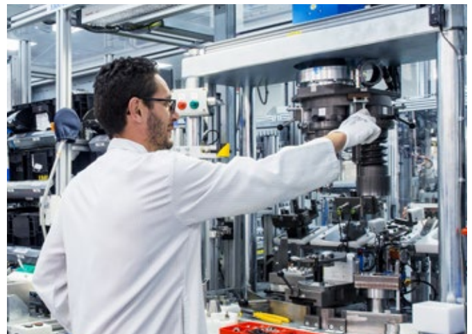
Assembly of common rail systems in the cleanroom
