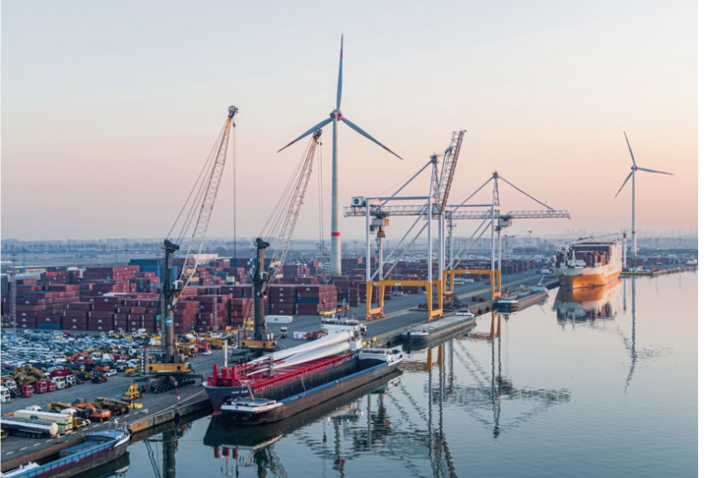
Two LHM 550 mobile harbour cranes in tandem lift operation at the Antwerp Euroterminal (Belgium)
