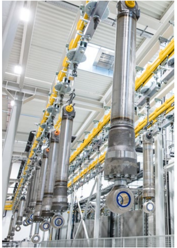
Robotised coating line for hydraulic cylinder series-production ranges
