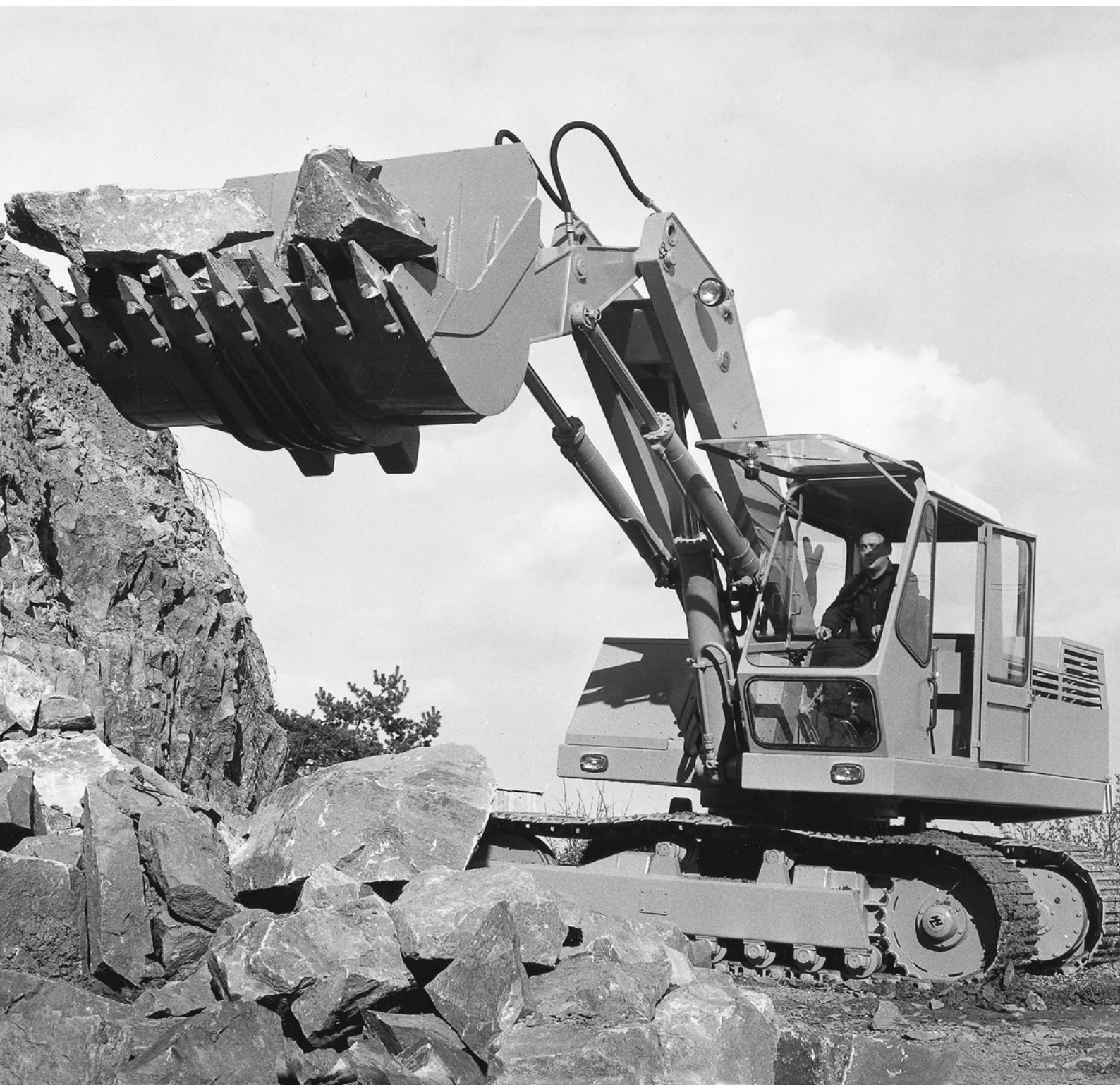
The Liebherr 20 t crawler excavator RT 100 from 1996 was equipped with a 130 HP/65 kW engine.
