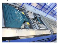
liebherr-air-cycle-air-conditioning-system-on-board.jpg - © Liebherr Liebherr demonstrator installed on an SNCF regional train (TER).
