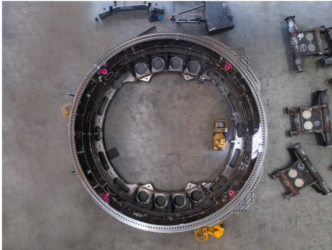
Crane in production: Just 14 metres is the diameter of the slewing unit of the HLC 150000-3000.
