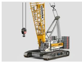
liebherr-lr 1250 unplugged\_1.jpg liebherr-lr 1250 unplugged\_2.png LR 1250.1 unplugged. – the world's first battery-powered crawler crane.
