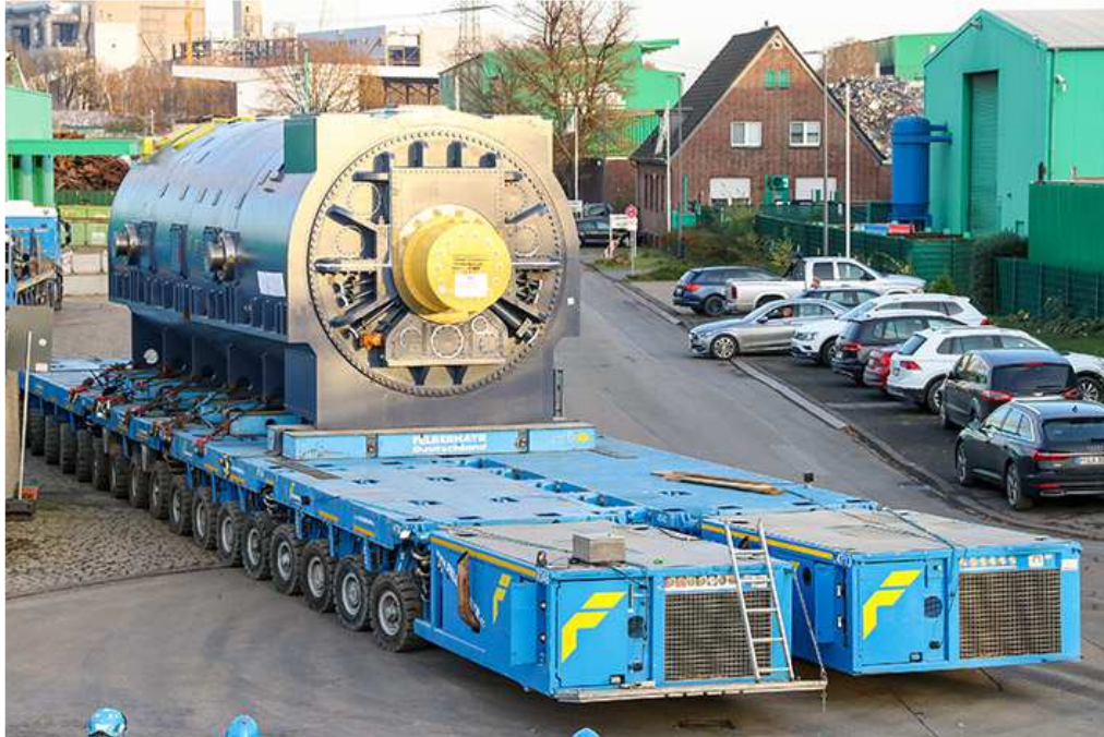
liebherr-felbermayr-lr11000-photo4.jpg Two SPMTs with 18 axles each take the generator to its operating location.
