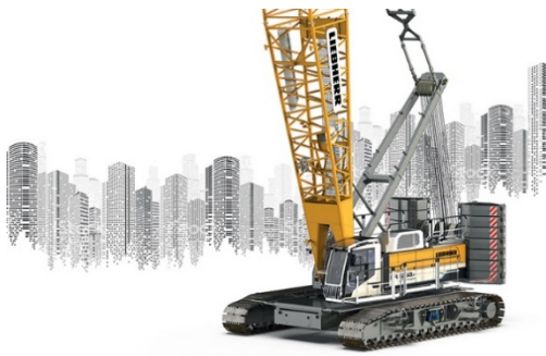
liebherr-Ir 1250 unplugged.jpg The world's first battery-powered crawler crane.
