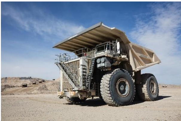
Liebherr-T274-mining-truck.jpg The T 274 is a true 305 tonne machine that provides fast cycle times, higher production rates, low fuel consumption, and a low cost per tonne.
