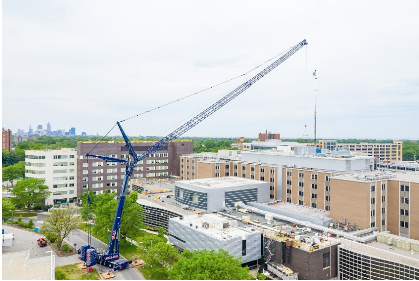
liebherr-all-kran-ltm1650-8.1-ohio1.jpg The new LTM 1650-8.1 from ALL on its first job in Ohio, US.
