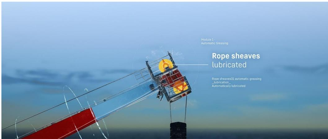
**Modul Automatic Greasing: Liebherr\_limain\_AutomaticGreasing.jpg**
