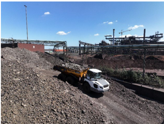
liebherr-earth-moving-machinery-report-heis-germany.jpg A TA 230 dump truck transports cooled slag from DK and piles it up.
