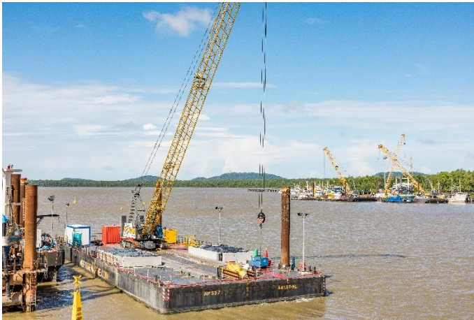
liebherr-usa-LR1100.1-crawler-crane.jpg The LR 1100.1 is powered by an efficient 230 kW diesel engine with a max load capacity of 110 USSt.
