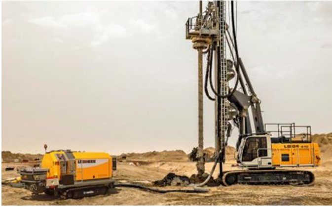
liebherr-usa-crawler-concrete-pump.jpg Liebherr THS 110 D-K crawler concrete pump with Liebherr drilling rig.
