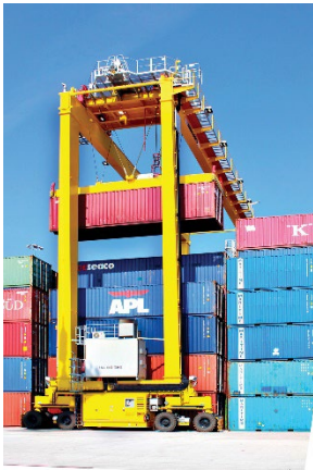
Liebherr-automated-rtg.jpg A cabinless Liebherr rubber tyre gantry crane (RTG)
