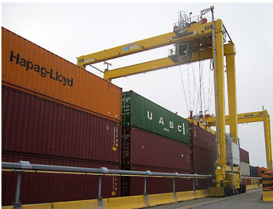
Liebherr-ERTG.jpg A busbar powered electric rubber tyre gantry crane (ERTG)
