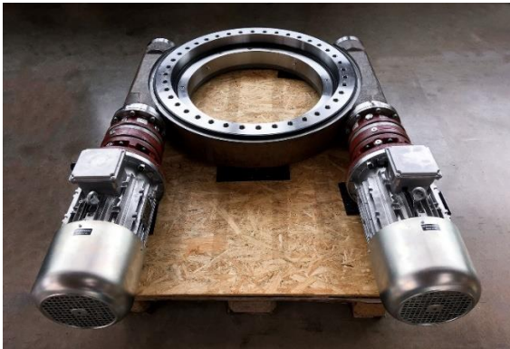
liebherr-slew-drives.jpg This slew drive by Liebherr is equipped with an electric motor.
