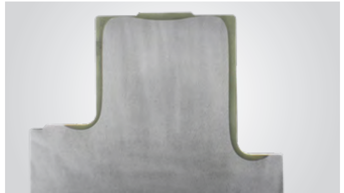
Grinding pattern of a roller bearing slewing ring with hardened
