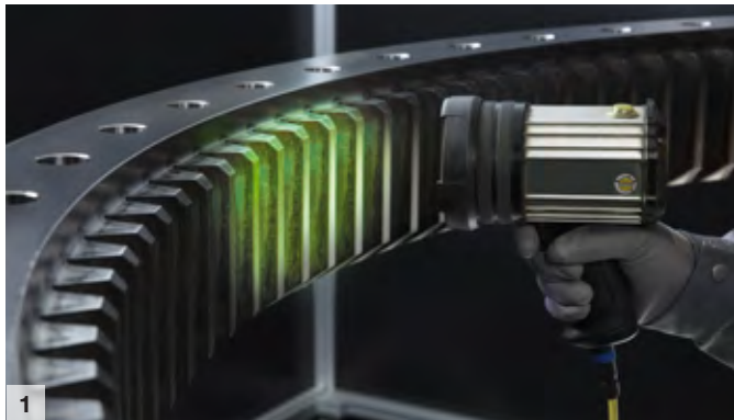
1 Magnetic particle inspection
