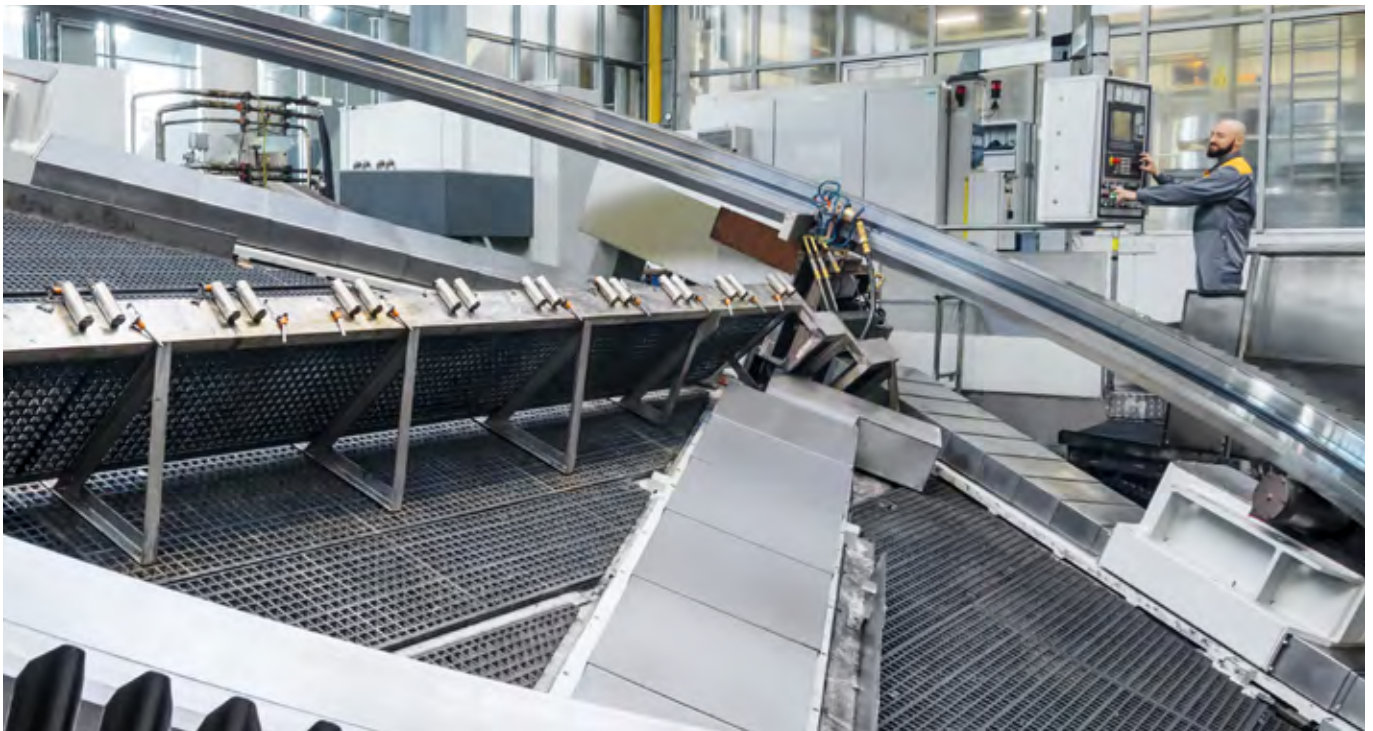
Induction hardening at Liebherr
