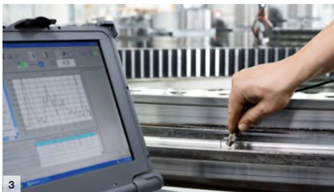
3 Measurement of hardness depth
