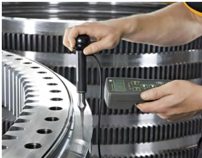
Quality check of slewing bearings
