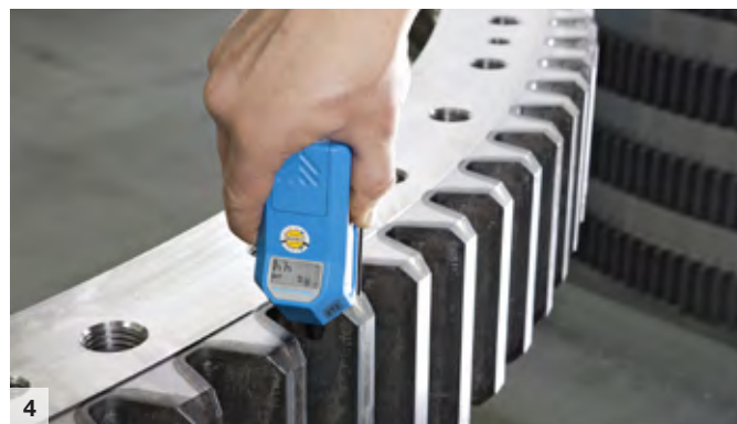
4 Surface inspection (surface roughness)
