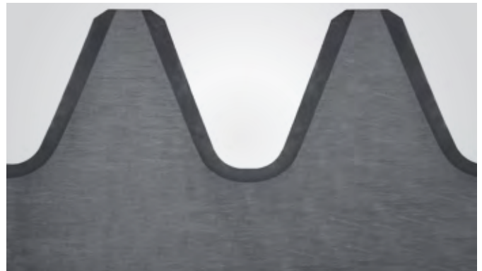
Hardening microsection of tooth spacing hardening
