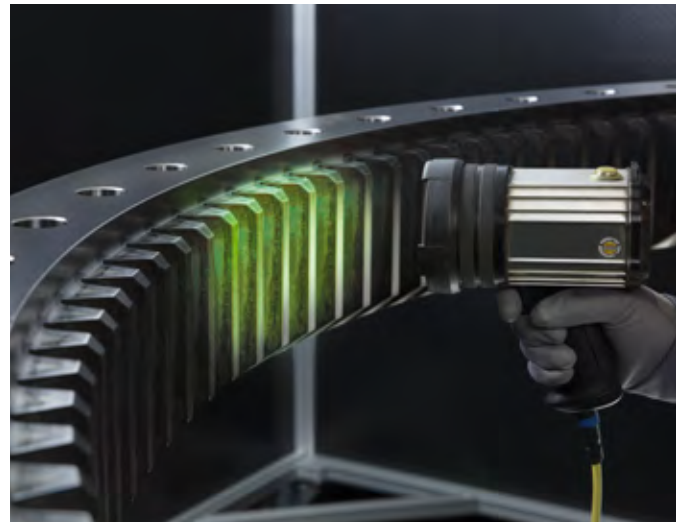
Quality check of slewing bearings using UV light
