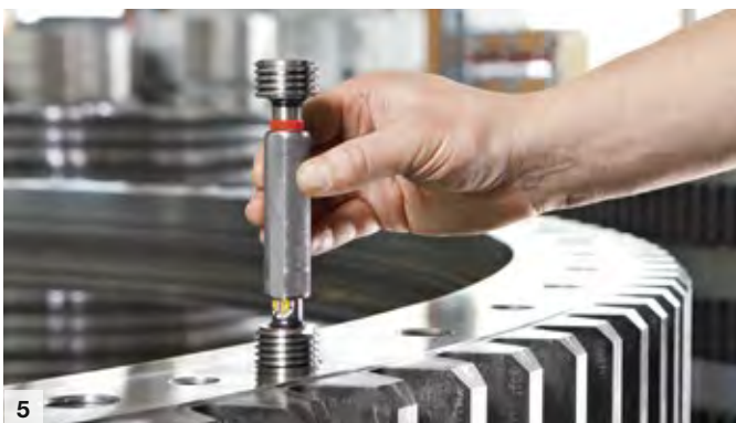
5 Dimension checks and visual inspection
