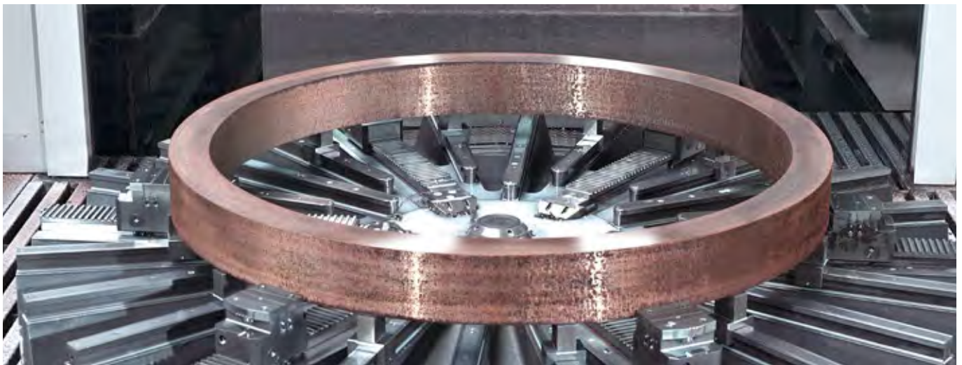
Rolled ring on turning machine
