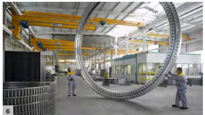
6 Completed large diameter bearing
