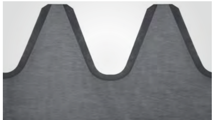
Hardening microsection of tooth spacing hardening
