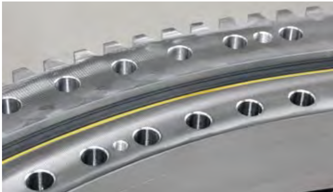
Built-up grease collar at the bearing seal
