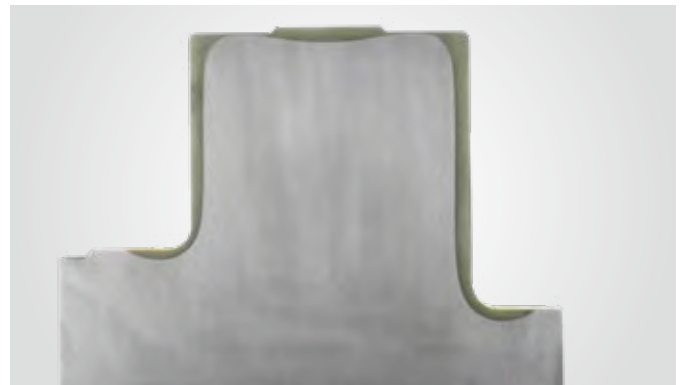
Grinding pattern of a roller bearing slewing ring with hardened case
