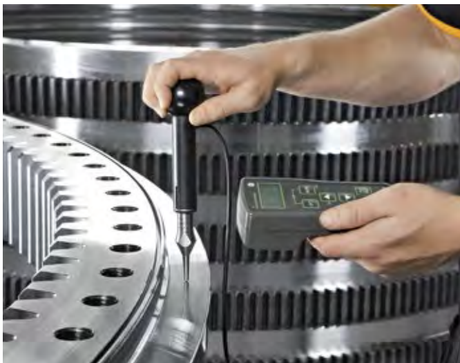
Quality check of slewing bearings
