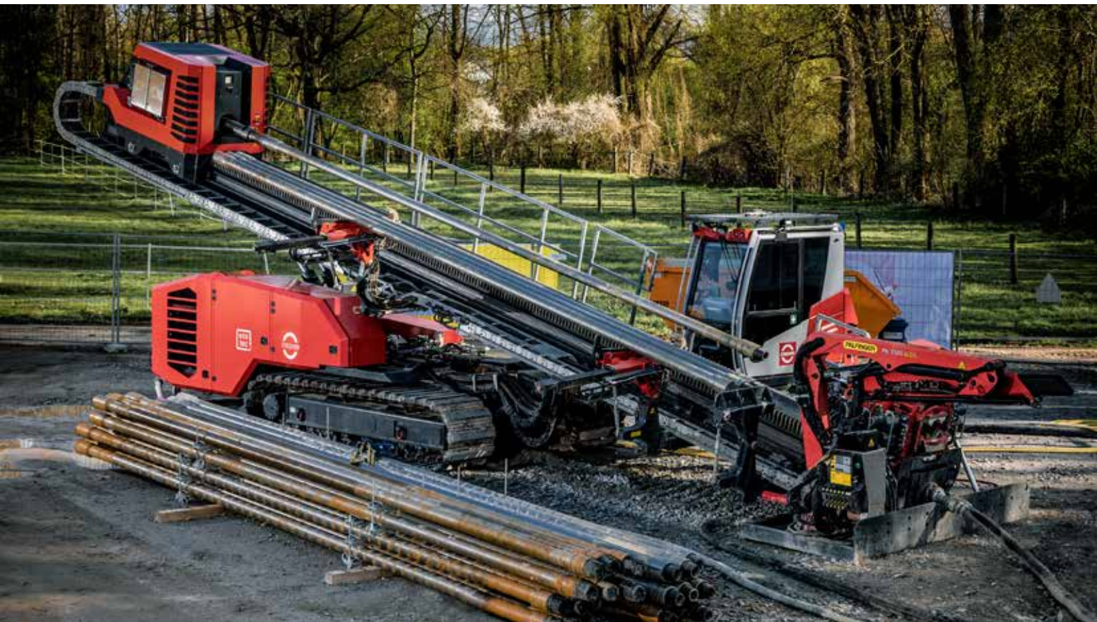
HDD drilling rig (horizontal directional drilling)
