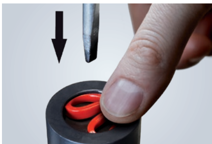
4. Press sealing disc down as far as the groove, position the screwdriver in the centre of the sealing washer and remove finger.
