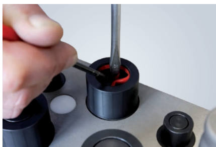
2. Press down sealing disc on the coupling plug with a screwdriver and remove the top sealing washer (red) with a sharp tool.
