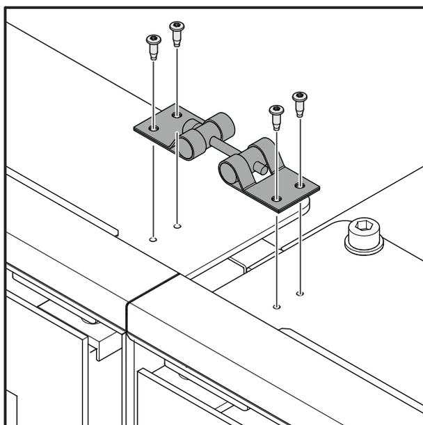
**B) Block configuration [torque 4-5 Nm]**
