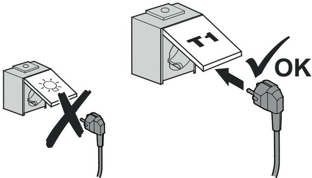
2. Plug the mains plug of the light cable into the appropriate socket.
