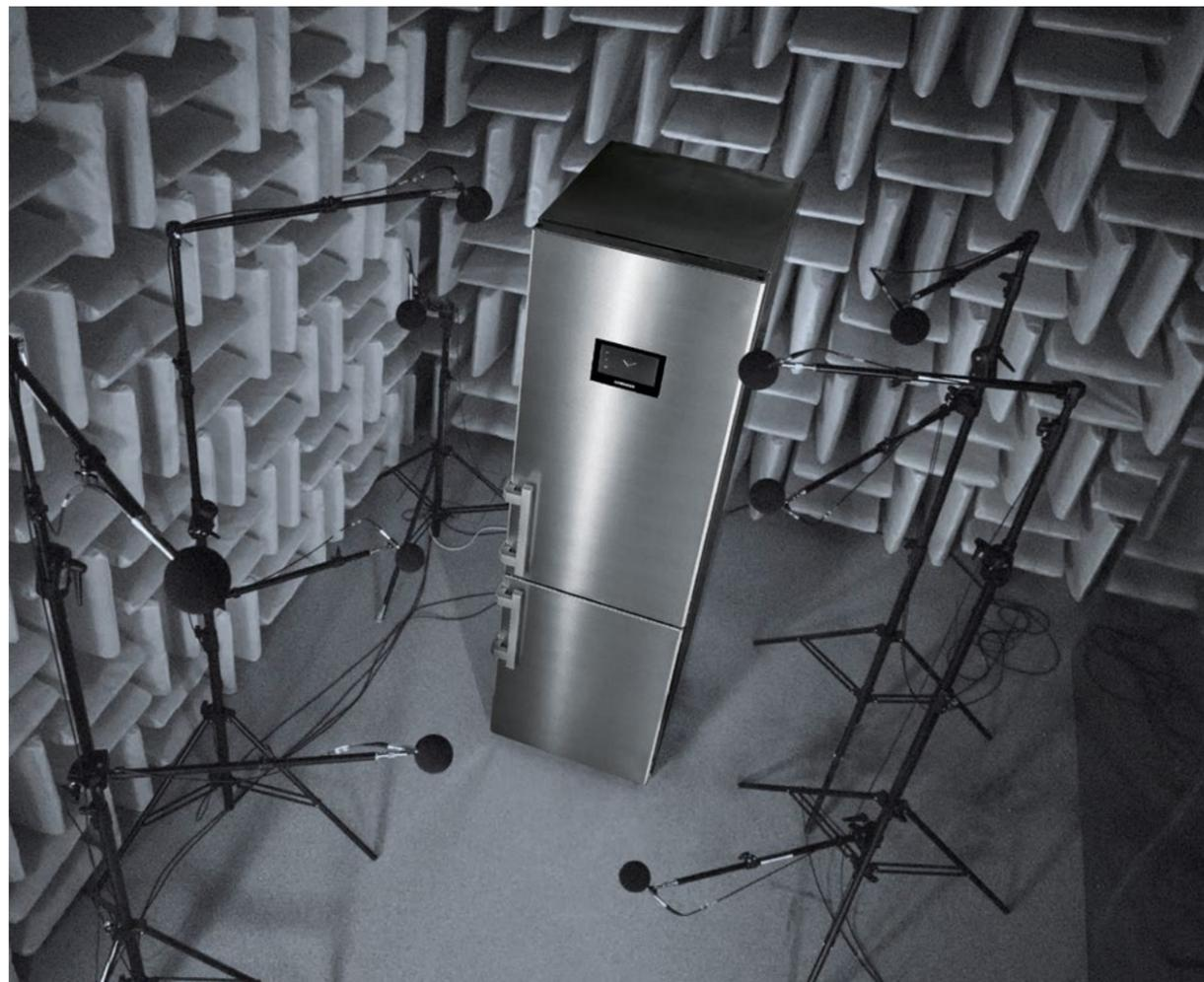
In professional sound measurement rooms, engineers use highly sensitive microphones to listen very carefully to sound emissions and further optimise the sound quality of moving components such as doors and pull-outs
