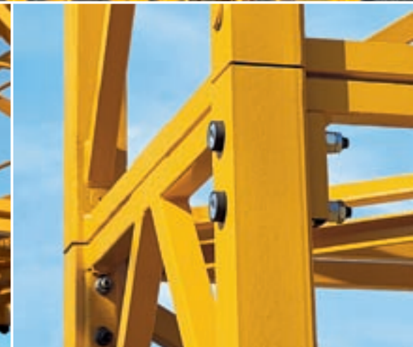
Liebherr's zero-clearance taper-pin connection for large cranes.
