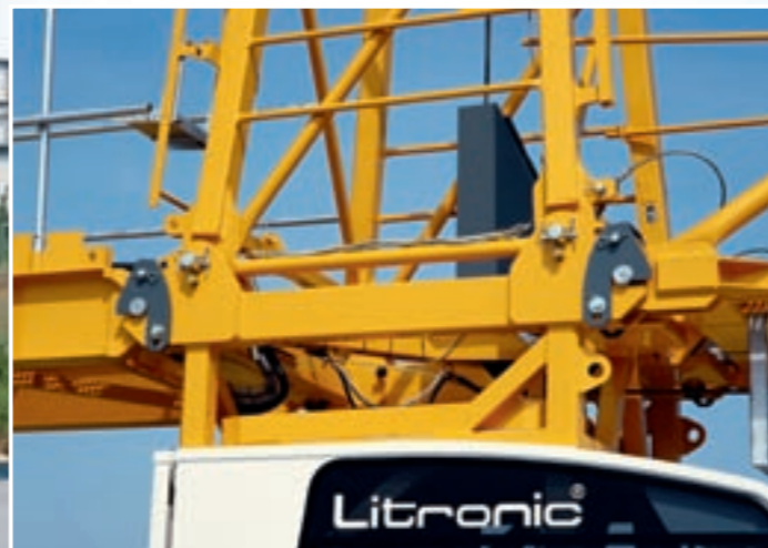
Quick-release fastenings for the jib and counter-jib.
