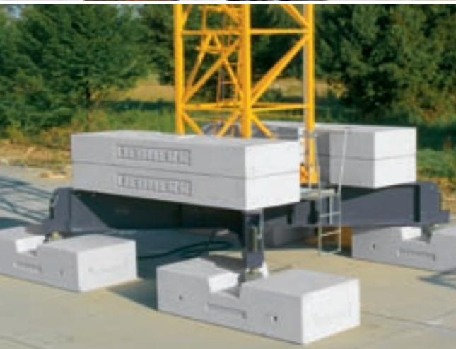
The stationary cruciform base with foundation blocks.
