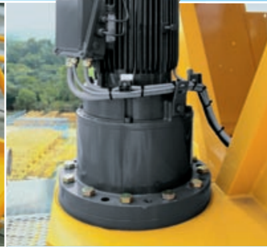
Patented frequency-converter slewing gear: sensitive, jerk-free slewing movements.
