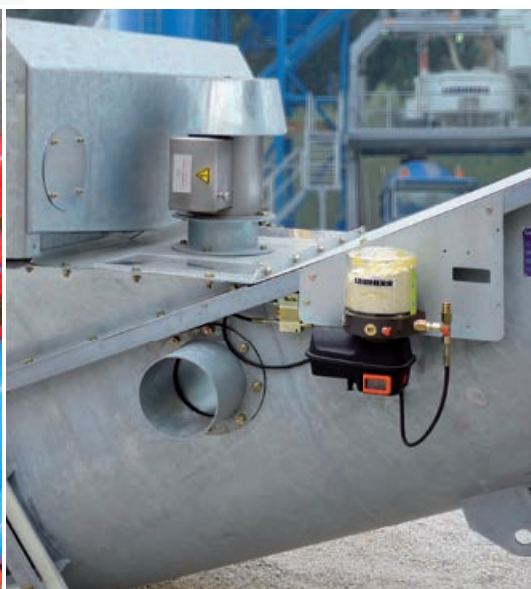
Heating (optional) and central lubrication system
