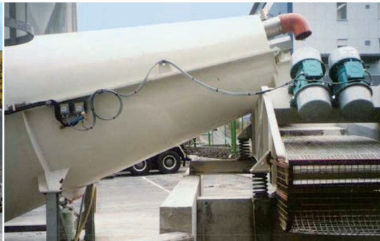
Separation of sand and gravel
