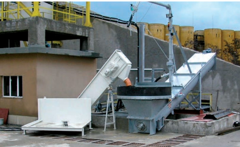
Conveyor with loading hopper
