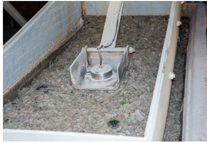
In sliding shoe for cullet (recycling glass)
