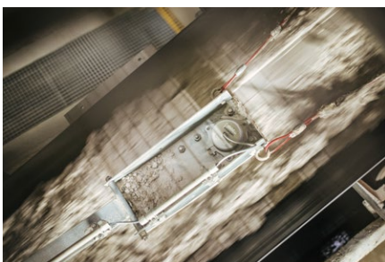
In sliding shoe for quartz sand (glass, building material and ceramic industry)
