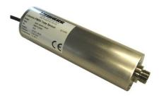
The Litronic FMS RMH12 pipe sensor is a so-called "intelligent sensor", i.e. the internal microprocessor enables complete problem-solving within a single component as well as extended functionality. The sensor transfers all of the relevant factory calibration data to the evaluation and transfer module 8 s after being switched on and following this transfers capacity raw value and both temperatures 30 times per second.
