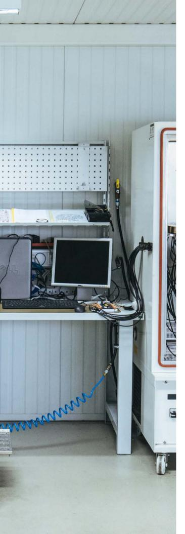
Since 1985 Liebherr develops, produces and distributes efficient moisture and water content measurement systems for the industrial automation around the world. At the Liebherr factory in Bad Schussenried the sensors are produced and calibrated in an ESD-protected production line. Each sensor will be tested separately in a several hour process across the entire working temperature range before leaving the factory.
