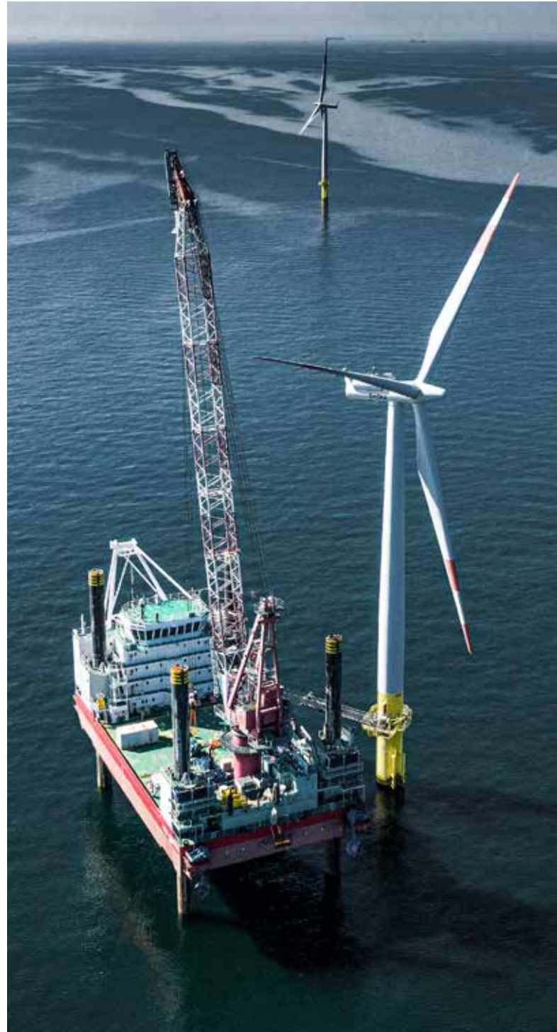
Offshore heavy-duty cranes have load capacities of up to 5,000 tonnes.
