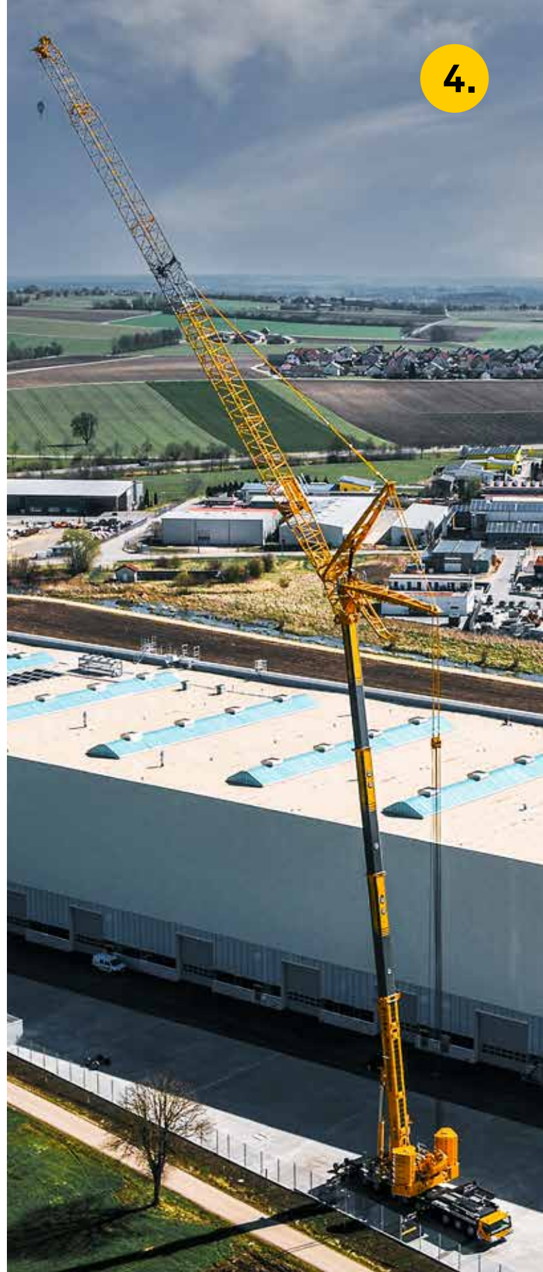
Cantilever The NK system requires the luffing jib to be guyed on the NK intermediate section.
