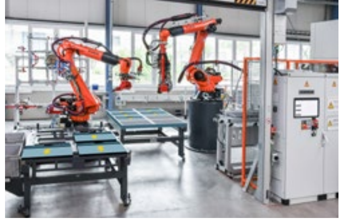
Liebherr pilot plant for the automated disassembly of battery packs
