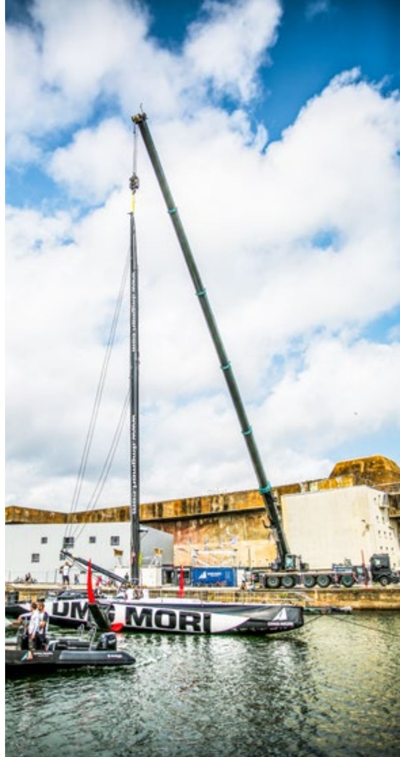
The LTM 1110-5.2 mounts the 29-metre long carbon masts on a total of 34 racing sailboats.
