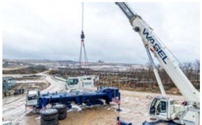
Final assembly: the final assembly of the LTL 1160 after its general overhaul in 2024 took place on site at the Hambach open-cast mine.
