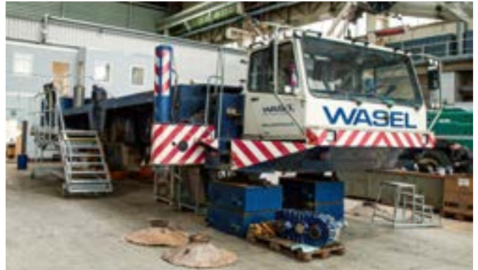
Dismantled down to the skeleton: the specialists from Liebherr completely dismantled the all-terrain crane for the general overhaul.
