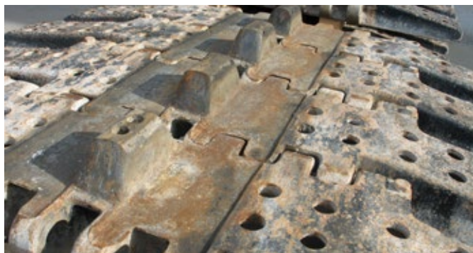
Ground plates with wear
