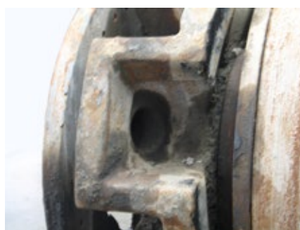
Wear on the sprocket
