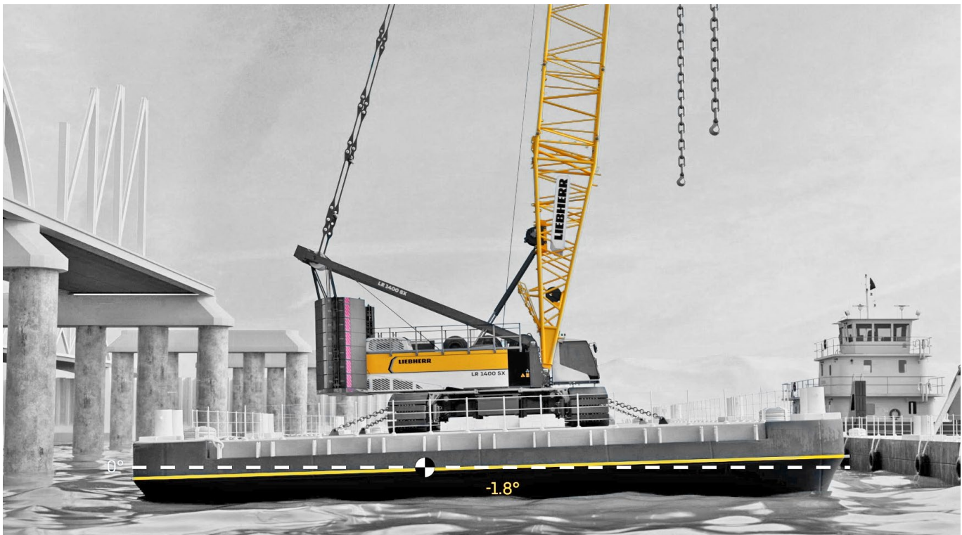
The inclination of the floating unit is monitored by the crane control system. Accordingly, the driver is warned if the set inclination angle is exceeded.
