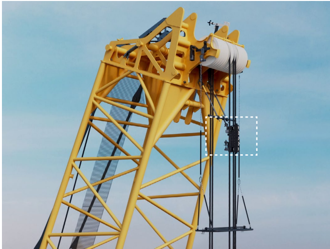
Sensors determine the rope lead-off angle
