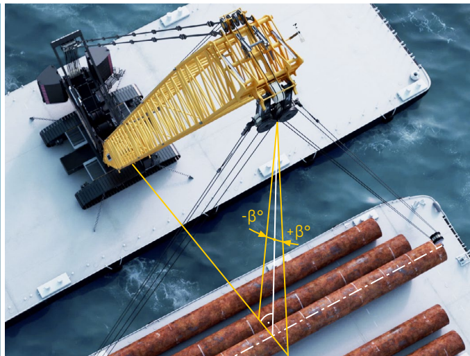
Optional Off-lead Compensation: At the touch of a button, the diagonal pull in the boom direction and thus the load swing in the boom direction can be avoided.
