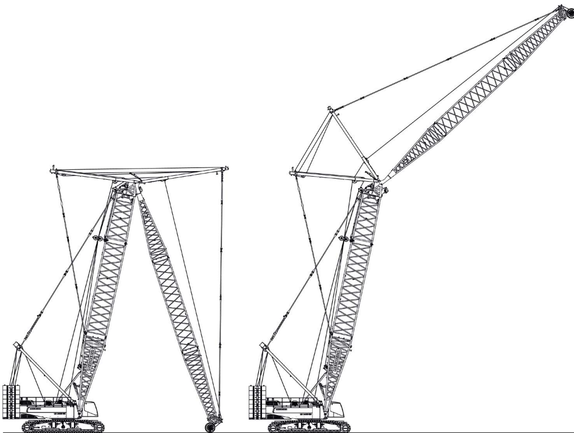
Erecting of main boom and luffing jib
