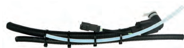
Fig. 49: Securing air line with cable ties
