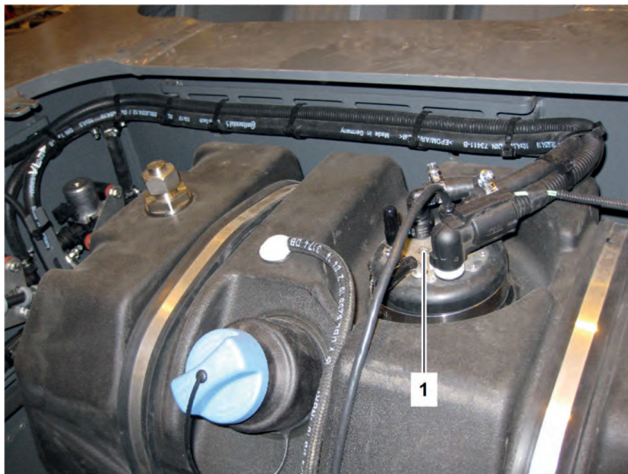
Fig. 58: Installed suction module
