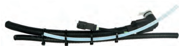
Fig. 54: Securing air line with cable ties
