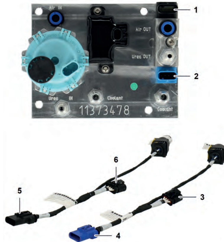
Fig. 66: Urea pump and cable harness
