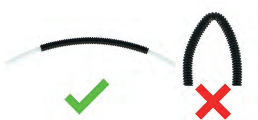
Fig. 53: Correct bending radius
