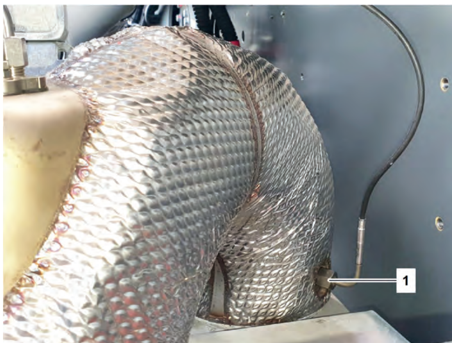
Fig. 73: Installed temperature sensor
