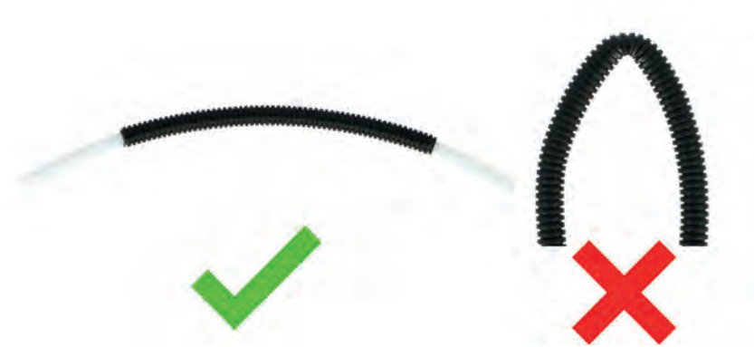
Fig. 48: Correct bending radius
