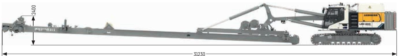
For maintenance and service work on the leader and carrier machine, the leader can be folded forward. In this position the piling rig cannot move or travel.
