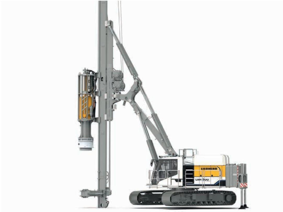
By supporting the leader on the ground and extending the rear support cylinders, the carrier machine is elevated. The undercarriage can thus be swivelled on the spot, which makes it easier to move the piling rig in restricted spaces.
