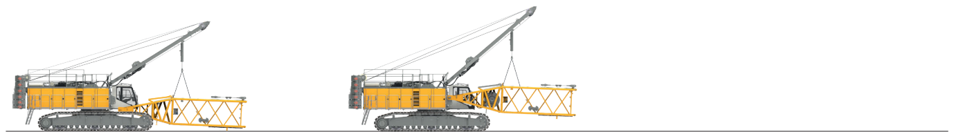
Assembly of boom foot
