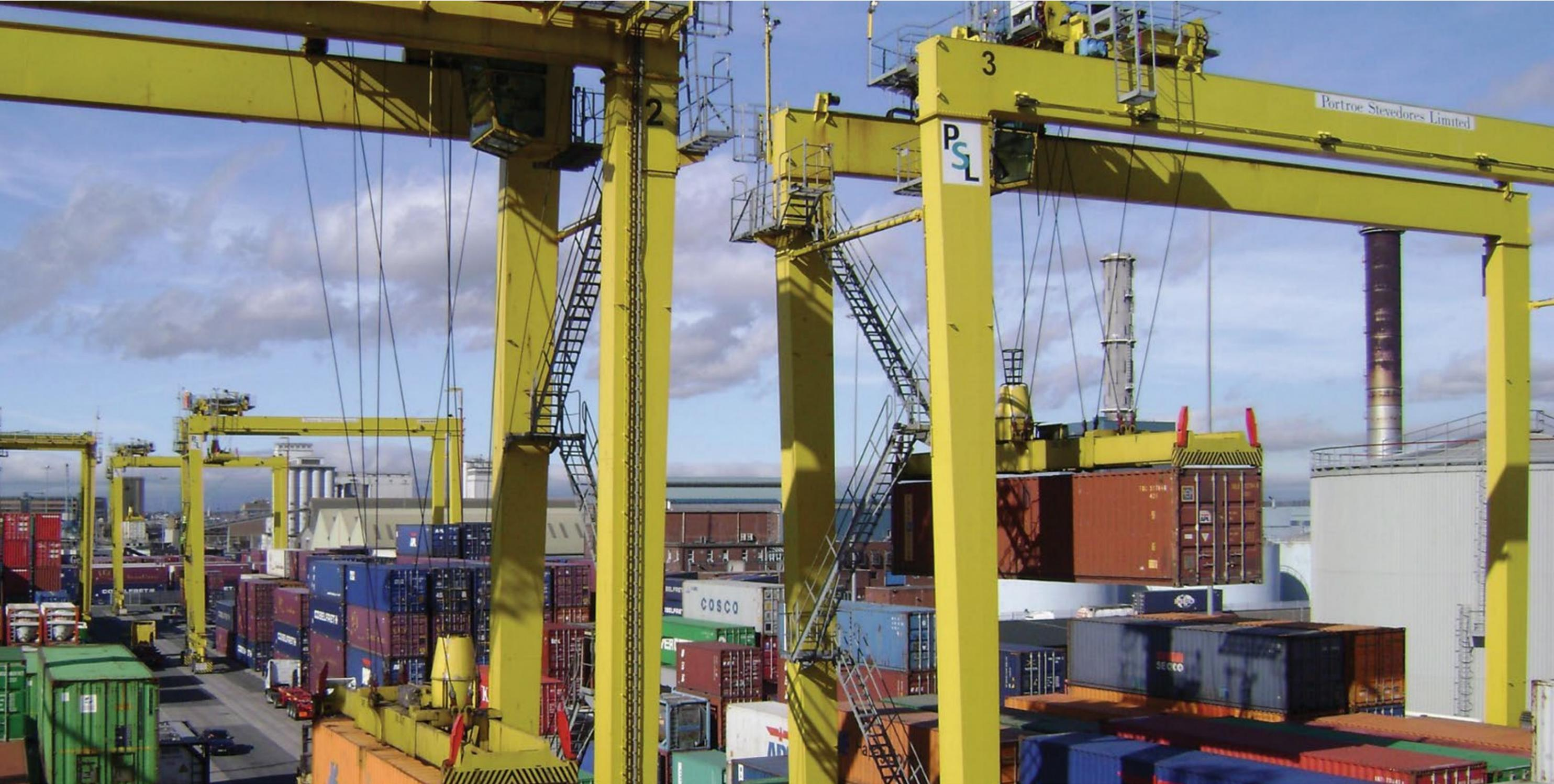
Liebherr RTGs feature an eight rope reeving anti-sway system and simultaneous drive motion of all drives. With increased productivity levels when compared with alternative designs, overall capital investment and costs per box handled are substantially reduced.
