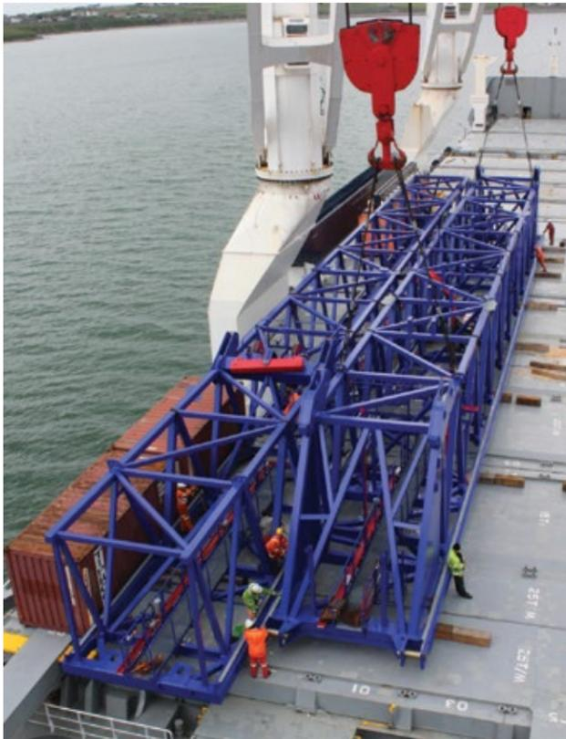
Liebherr has extensive experience in shipping of cranes to all parts of the world. All cranes are exported through the nearby Port of Fenit. In order to speed up the on-site installation, crane sections are assembled and tested to the maximum extent possible, prior to loading on to the delivery vessel.
