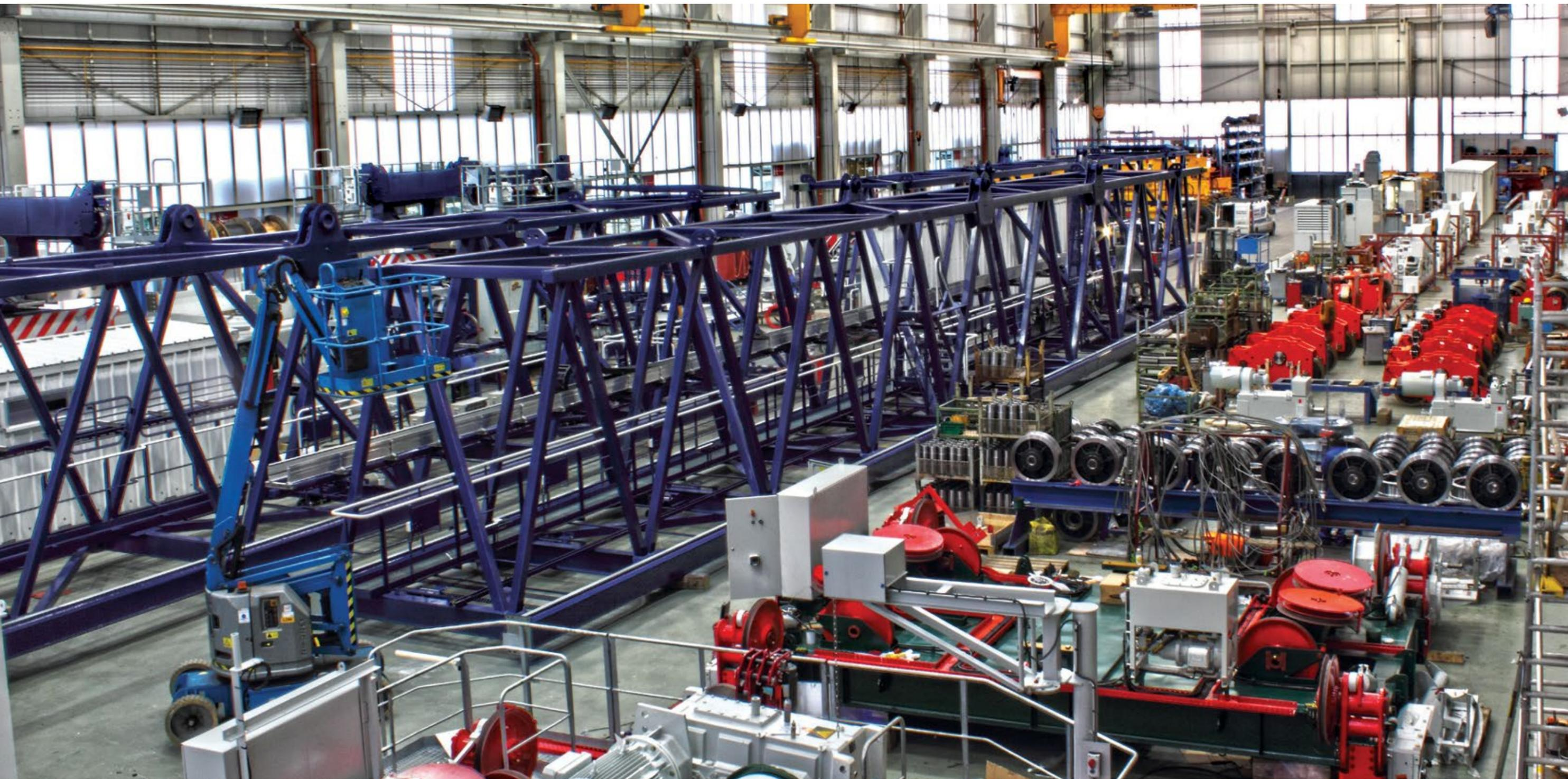
Before a crane is dispatched, all electrical and machinery houses are assembled and electrically connected prior to testing. Container crane and RTG gantry bogies are assembled. Main beams and booms are equipped with cabling, lights etc. Trolleys and cabins are assembled, wired and tested, ready for shipping. Extensive testing in final assembly ensures a fast and efficient installation.
