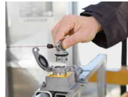
Access secured by a limit switch
