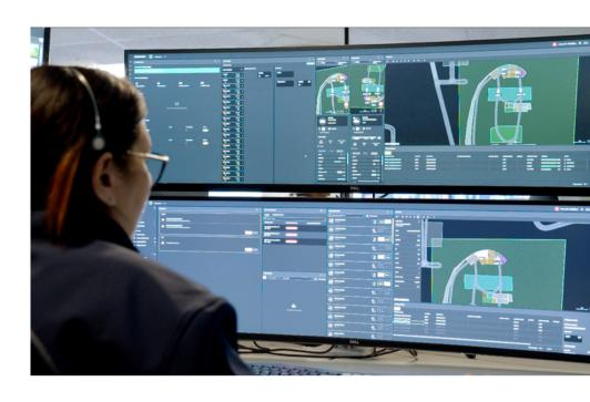
The Autonomous Haulage Solution (AHS) enables the completely autonomous operation of our haul trucks by combining advanced automation with real-time data insights to enhance productivity, safety and efficiency. This solution is what will be installed onto the T 264 battery-electric truck to make it an autonomous battery-electric truck.
