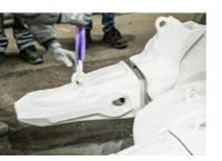
**Step 1:** Insert the tooth into the adapter.
