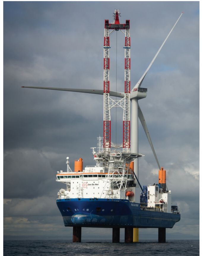
This CAL 45000 offshore crane, which is designed as a crane around the leg, in operation on-board the 'Vole au Vent', can lift up to 1,200 tonnes.
