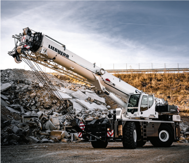
47 meter telescopic boom, a maximum hook height of 66 meter and a maximum load capacity of 90 tonnes characterise the LRT 1090-2.1.
